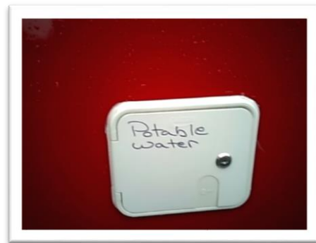
Potable Water Inlet
